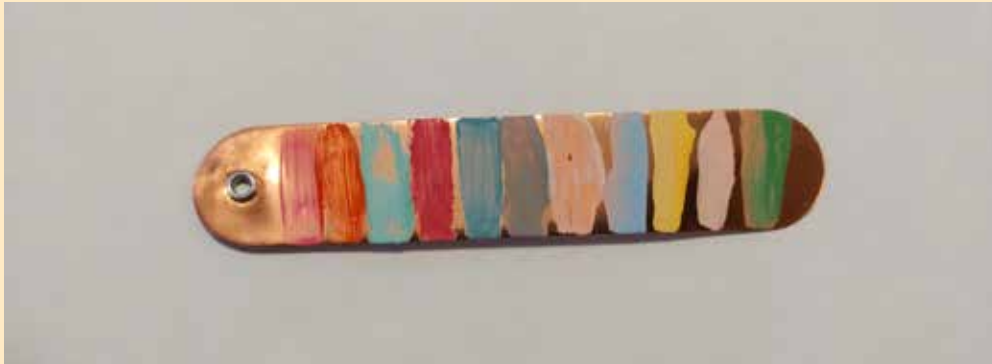
Pyrometer, made in the lab to record fire intensity in the field
